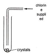
When more chlorine is added and the tube is sealed, a reversible reaction occurs and the reaction comes to equilibrium.
