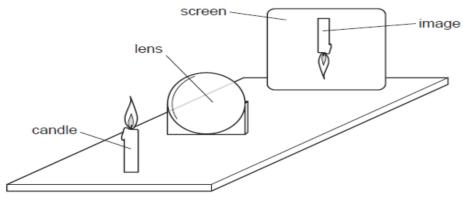
Various focused images are produced on the screen by moving the lens and the screen backwards and forwards.
