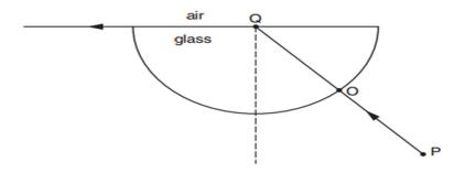
The ray of light PO hits the glass at O at an angle of incidence of 0°. Q is the centre of the straight side of the block.
