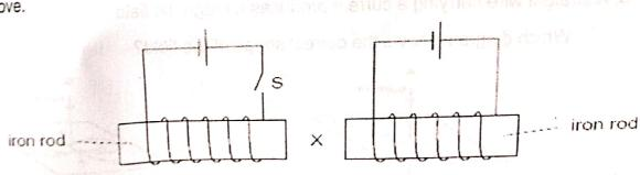
What happens to the size of the gap at X when switch S is closed?
