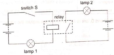
When switch S is closed, the relay operates. What is the state of the lamps?
