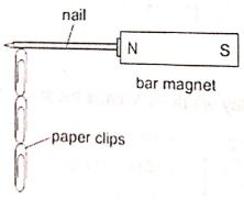
One of the nails is placed against a bar magnet and the number of paper clips which the nail can support is recorded. The bar magnet and the number of paper clips which the nail can support is recorded. The bar magnet and the number of paper clips remaining attached to the pail is a removed and the number of paper clips. clips remaining attached to the nail is recorded. Each nail is tested in turn.
