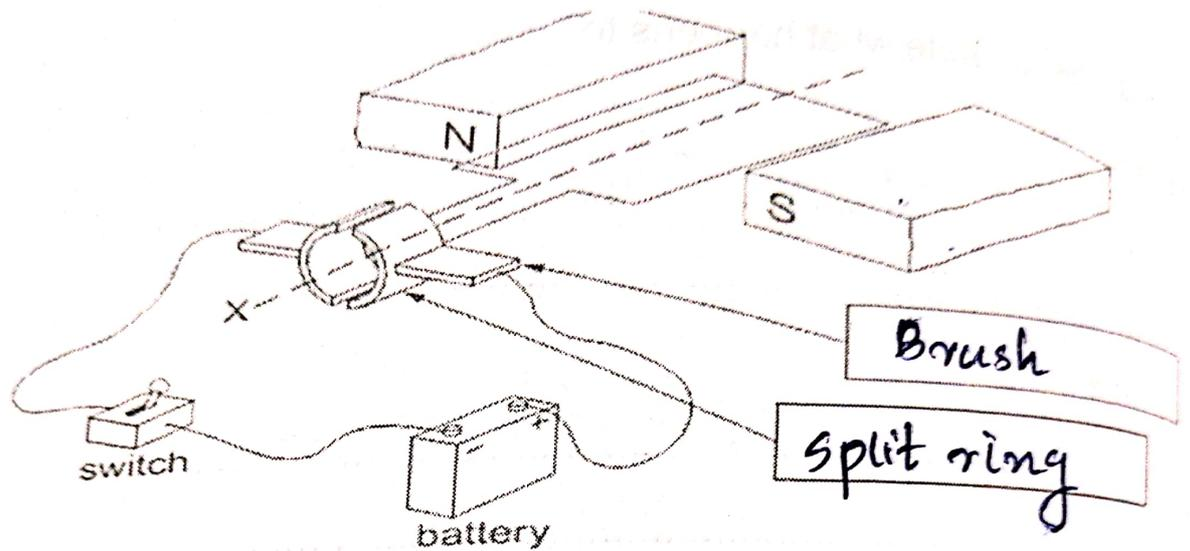
(i) On Fig. 9.2, write in each of the boxes the name of the part of the motor to which the arrow is pointing.
