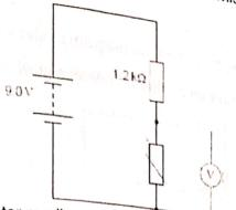
Calculate the voltmeter reading when the resistance of the thermistor is 3.6 k $\Omega$ .
