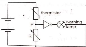
Explain, with reference to the components in the circuit and point P, (i) why the warning lamp is on when the temperature in the oven is below the set value,
