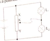
The contact K is halfway between X and Y and the lamps are equally bright.
