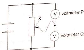
The sliding connection at point X is moved towards the top of the diagram.
